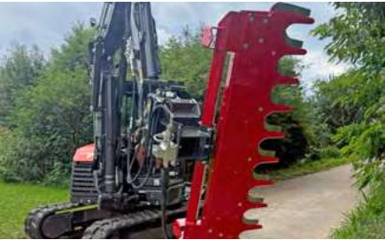
Boom extends 1200 mm to the side. Cutter bar made from highly wear-resistant steel HB 500
