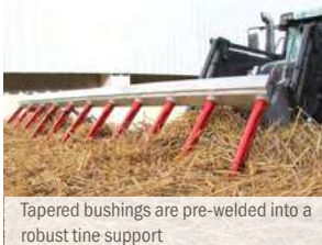
Robust scraper rail protects the bucket base
