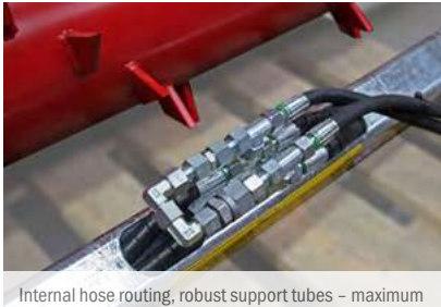
Internal hose routing, robust support tubes – maximum hose protection
