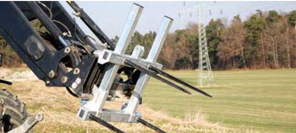
Version with extension and 4 round bale tines (2 tines as standard)
