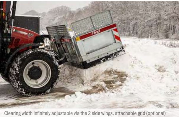
Clearing width infinitely adjustable via the 2 side wings, attachable grid (optional)
