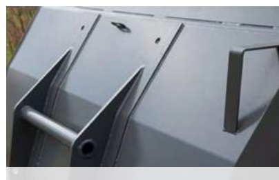
Orientation aid for horizontal loading of bulk materials
