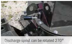
Discharge spout can be rotated 270°
