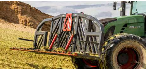
»Heavy-Duty« silage fork with blade attachment for corn silage
