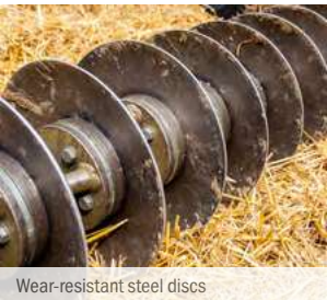
Wear-resistant steel discs
