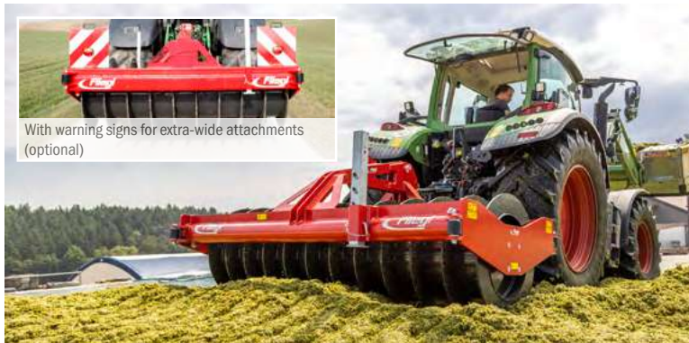
Silage roller double-sided adjustment
