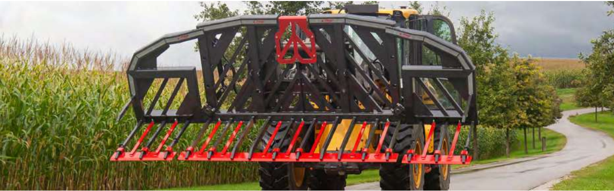
»Heavy-Duty« silage fork with blade attachment for corn silage
