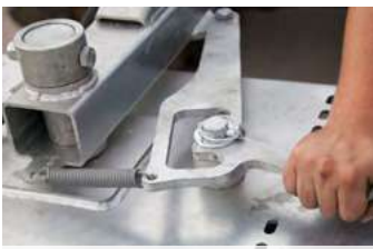
Mechanical swivel frame (30°), with optional hydraulic pivoting headstock
