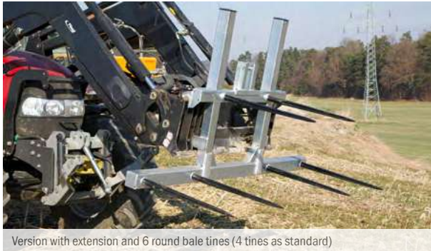
Version with extension and 6 round bale tines (4 tines as standard)
