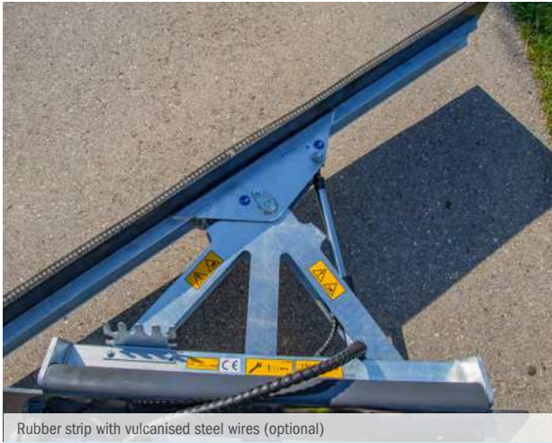
Rubber strip with vulcanised steel wires (optional)
