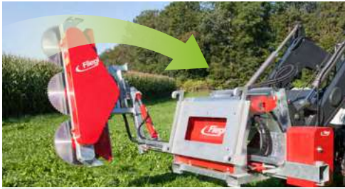
Swivelling pruning saw head for left and right attachment
