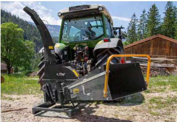
Opening angle of discharge flap adjustable
