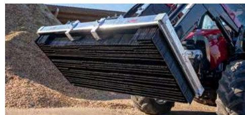
Replaceable brush rows and parking skids for gentle storage
