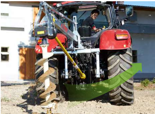
Wide swivel range, with drill (optional)
