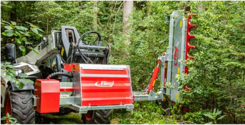
Boom extends 1200 mm to the side. Cutter bar made from highly wear-resistant steel HB 500
