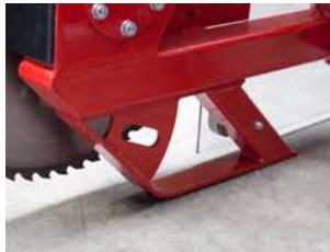
Guard rail prevents bottom saw blade from touching the ground.
