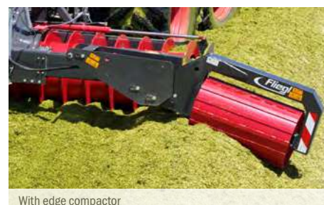
With edge compactor
