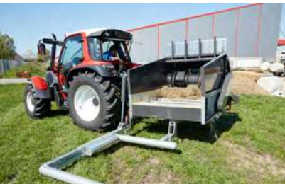
Hydraulic adjustment of gripping arm
