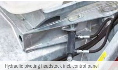
Hydraulic pivoting headstock incl. control panel
