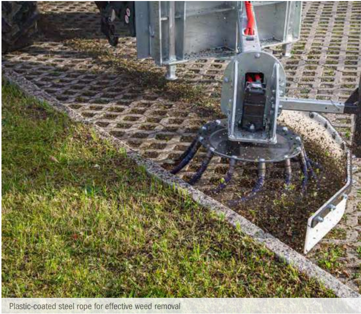
Plastic-coated steel rope for effective weed removal
