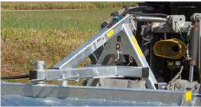
Three-point headstock for front and rear attachment
