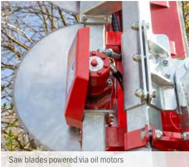
Saw blades powered via oil motors
