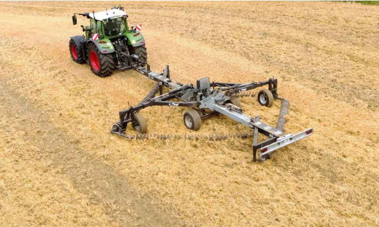
Heavy-duty chains with adjustable aggressiveness from 51° to 58°
