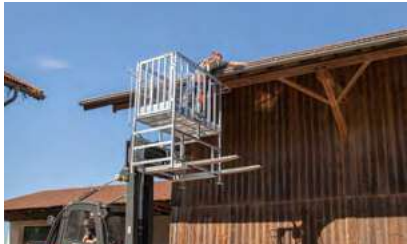
Attached to forklift with chain guard
