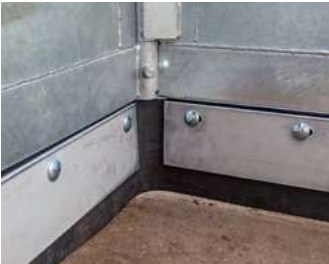
Rails made from steel HB 450
