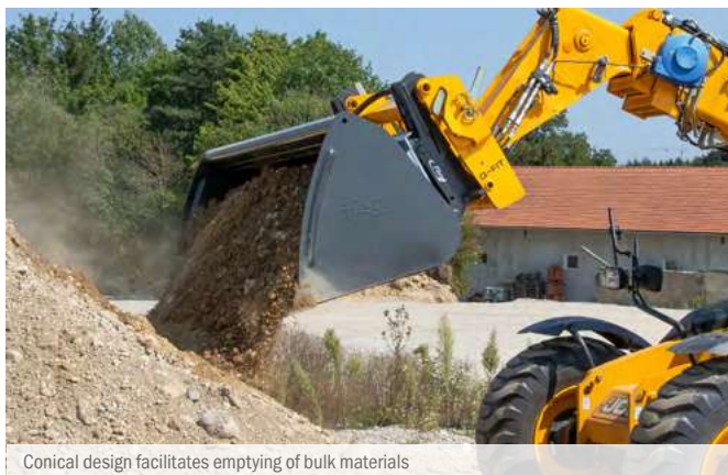
Conical design facilitates emptying of bulk materials
