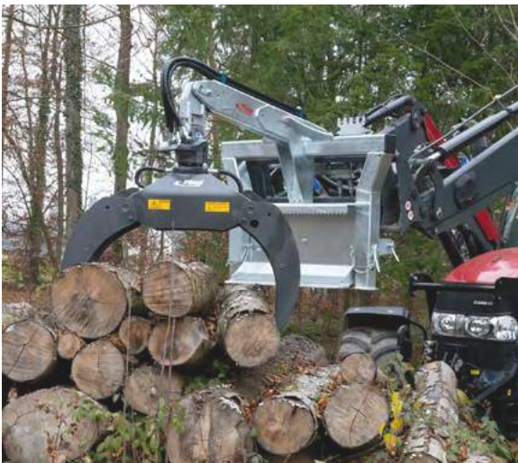
»RZ 185 Combi-Plus« hydraulic grapple with stacking blade (optional)
