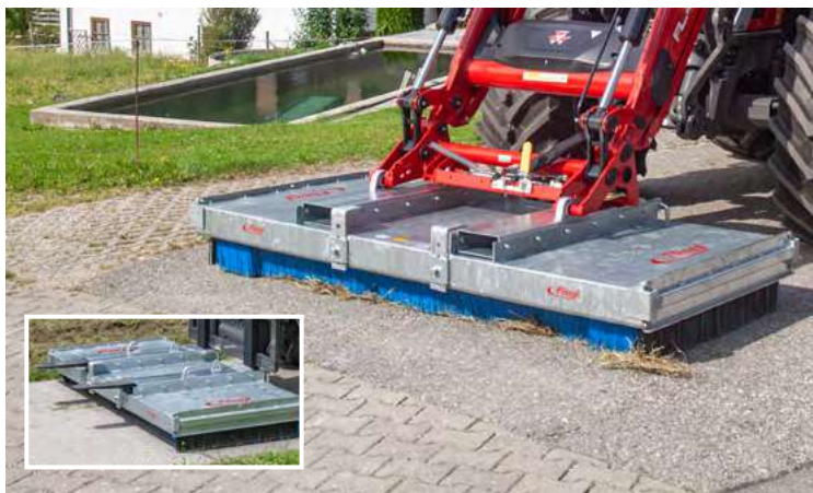
Combined Euronorm and forklift loader mounting
