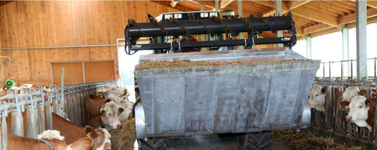
Feeding bucket, shown here with milling drum (not included with delivery)
