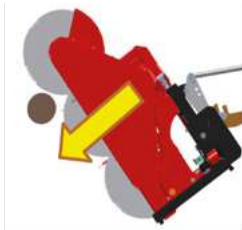
Note: Always cut thick branches from top to bottom to avoid jamming the saw blades!
