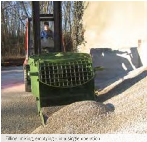
Filling, mixing, emptying – in a single operation
