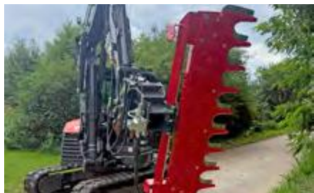
Boom extends 1200 mm to the side. Cutter bar made from highly wear-resistant steel HB 500
