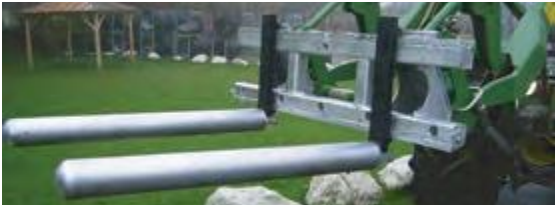
Attachable tubes for transporting round bales, secured with screws
