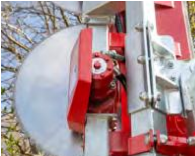
Saw blades powered via oil motors
