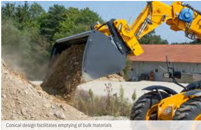
Conical design facilitates emptying of bulk materials
