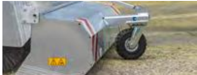
Heavy-duty support wheels Ø 306 mm – super-elastic solid rubber tyres, width 105 mm, ball-bearing mounted, wear-resistant tread, heavy-duty slewing ring design
