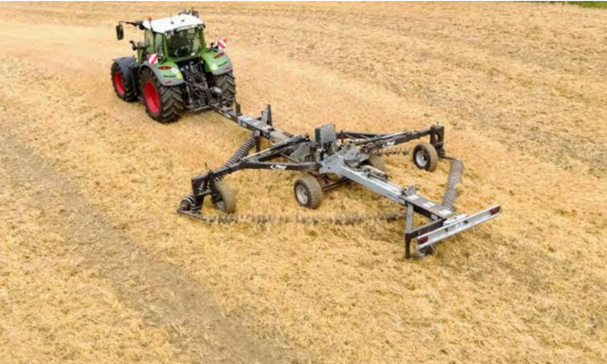
Heavy-duty chains with adjustable aggressiveness from 51° to 58°
