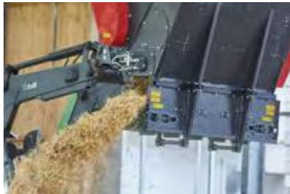
3 dosing rollers with blades
