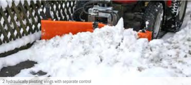
2 hydraulically pivoting wings with separate control
