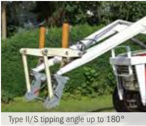
Type II/S tipping angle up to 180°
