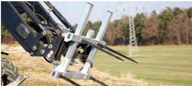
Version with extension and 4 round bale tines (2 tines as standard)
