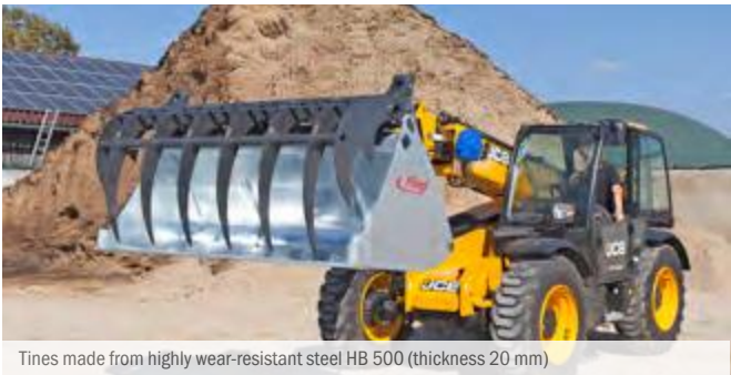
Tines made from highly wear-resistant steel HB 500 (thickness 20 mm)
