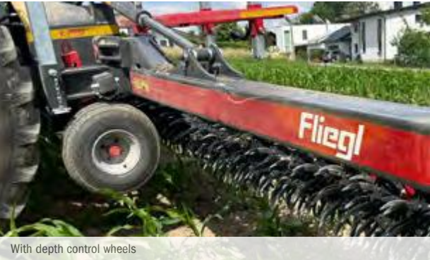
With depth control wheels
