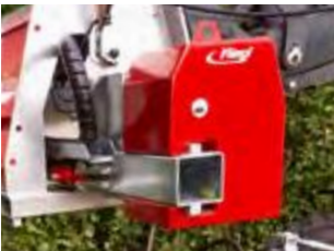
Lateral counterweight helps to reduce one-sided loads on the carrier vehicle linkage
