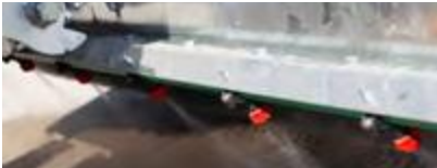
Spraying system – the splash guard nozzles are protected on the housing and spray the water close to the brush and prevent dust formation
