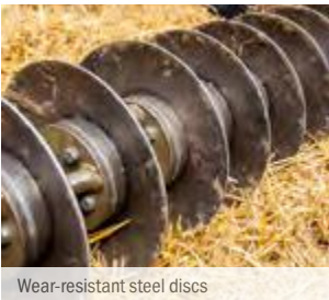
Wear-resistant steel discs
