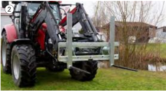
Adjustable mounting for round bale tines M28 x 1.5 mm
