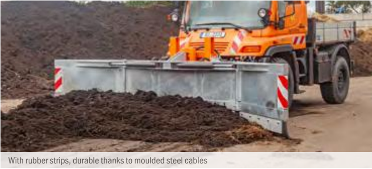
With rubber strips, durable thanks to moulded steel cables
