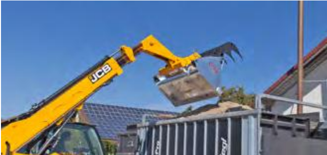
Tines made from highly wear-resistant steel HB 500 (thickness 20 mm)
