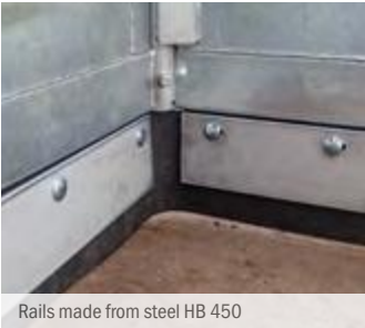
Rails made from steel HB 450
