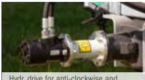
Hydr. drive for anti-clockwise and clockwise rotation
