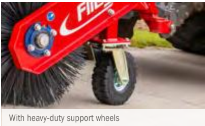
With heavy-duty support wheels
