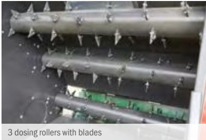
3 dosing rollers with blades
