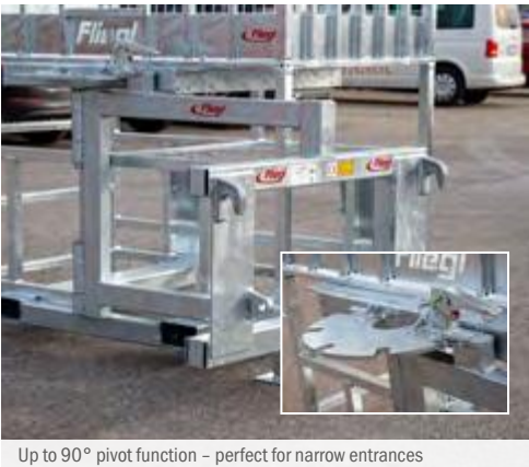
Up to 90° pivot function – perfect for narrow entrances
