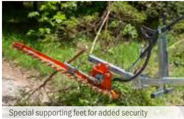
Special supporting feet for added security
