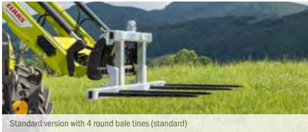
Standard version with 4 round bale tines (standard)
