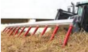
Tapered bushings are pre-welded into a robust tine support
