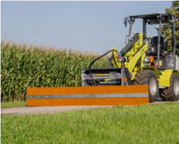
Rubber strip with vulcanised steel wires (optional)
