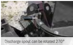
Discharge spout can be rotated 270°
