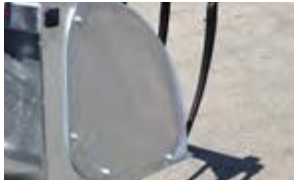
Bucket curvature with reinforced side walls increases stability
