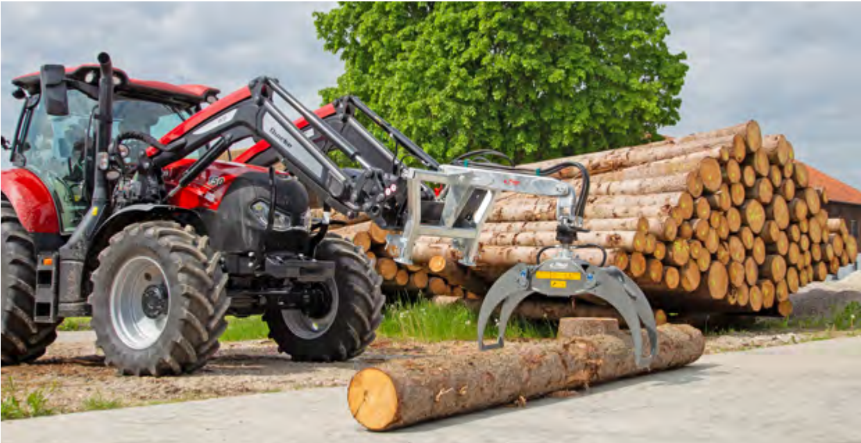
Loading gripper with load hook extension, rotary motor, Euronorm and three-point linkage
