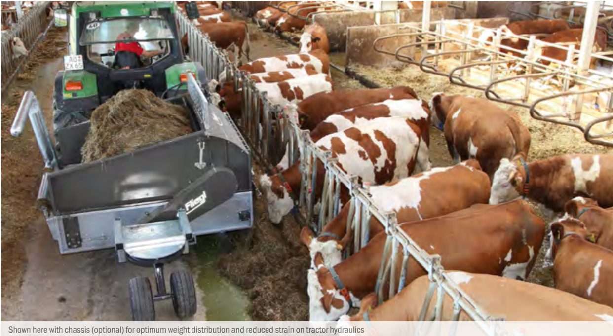
Shown here with chassis (optional) for optimum weight distribution and reduced strain on tractor hydraulics
