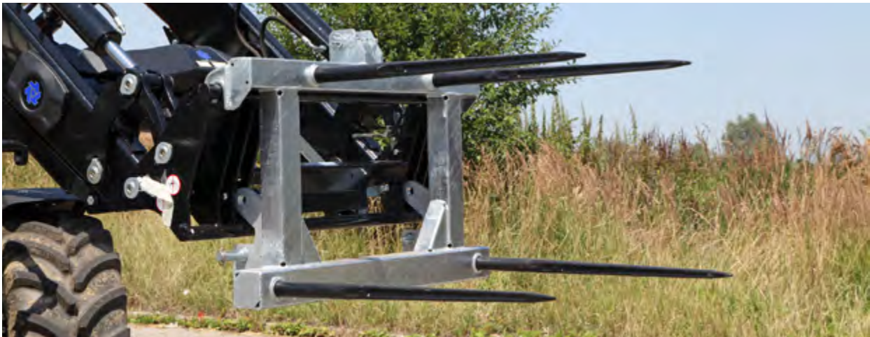
Standard version, shown here with 4 round bale tines (2 tines as standard)
