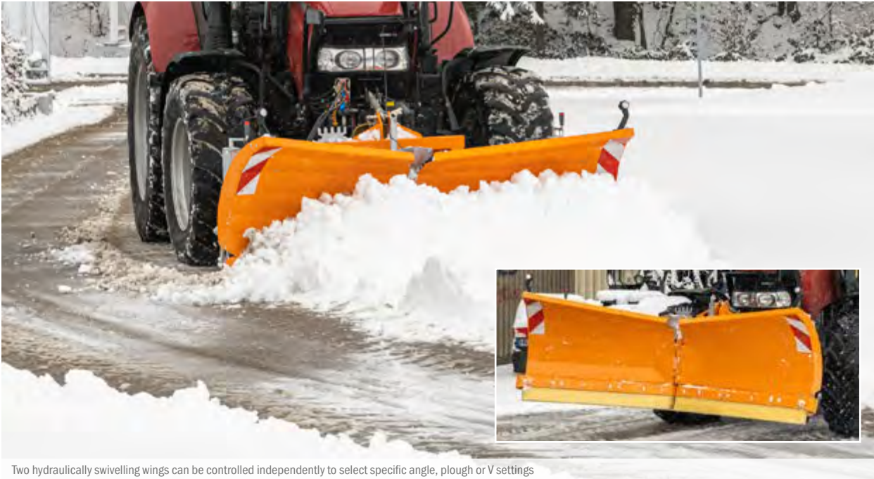
Two hydraulically swivelling wings can be controlled independently to select specific angle, plough or V settings
